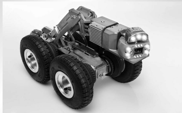
Crawler C 135 with camera KS 135 Scan HD
