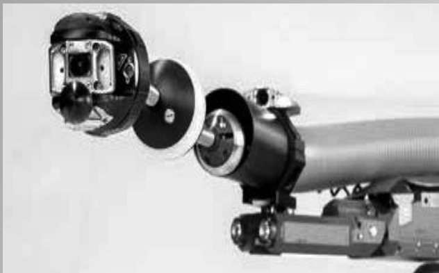
LATRAS sensor head with camera KS 60 HD and jetting system
