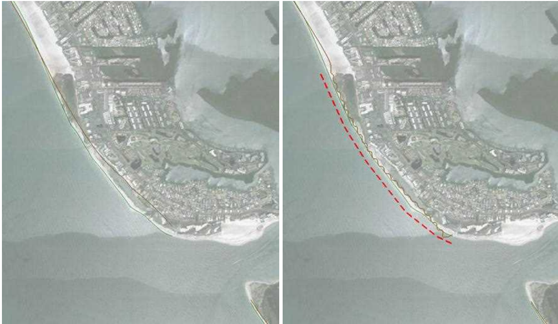
Figure 67. Beach response for Reach 3 for (left) FWOP conditions and (right) Alt 3.1 after 12 years. Green line represents the shoreline at year 0, and the brown line is the shoreline at year 12.
