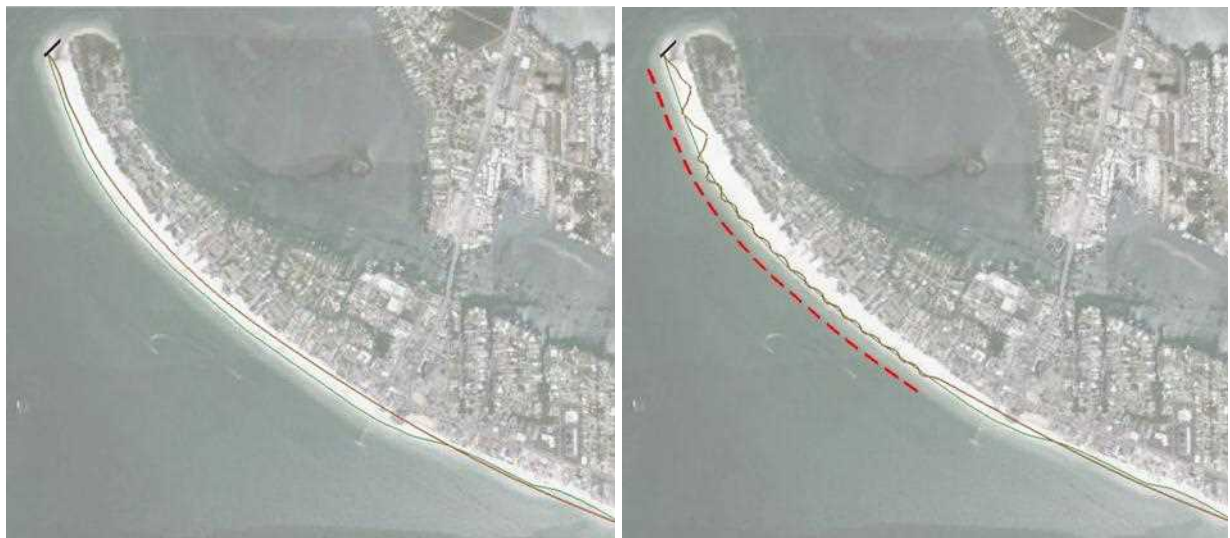
Figure 60. Beach response for Reach 1 for (left) FWOP conditions and (right) Alt 1.3 after 8 years. Green line represents the shoreline at year 0, and the brown line is the shoreline at year 8.
