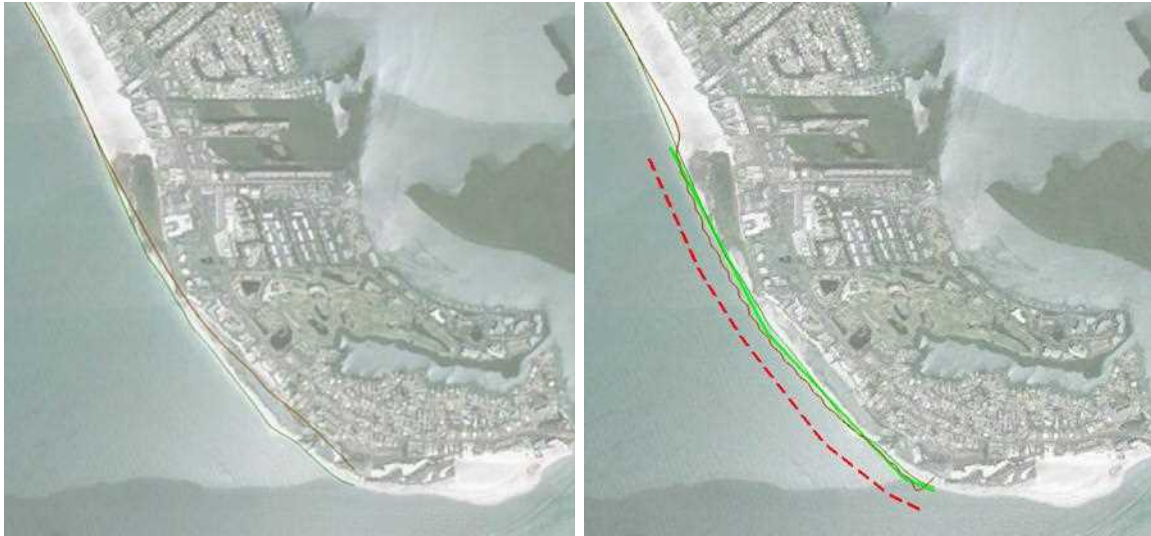
Figure 71. Beach response for Reach 3 for (left) FWOP conditions and (right) Alt 3.3 after 8 years. Green line represents the shoreline at year 0, and the brown line is the shoreline at year 8.
