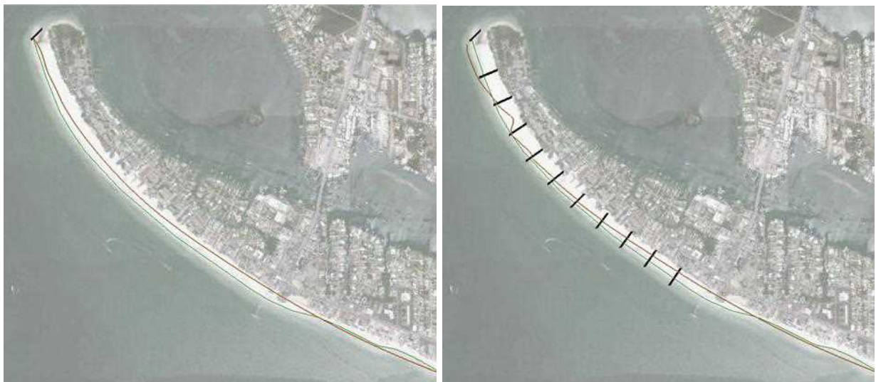
Figure 56. Beach response for Reach 1 for (left) FWOP conditions and (right) Alt 1.2 after 8 years. Green line represents the shoreline at year 0, and the brown line is the shoreline at year 8.
