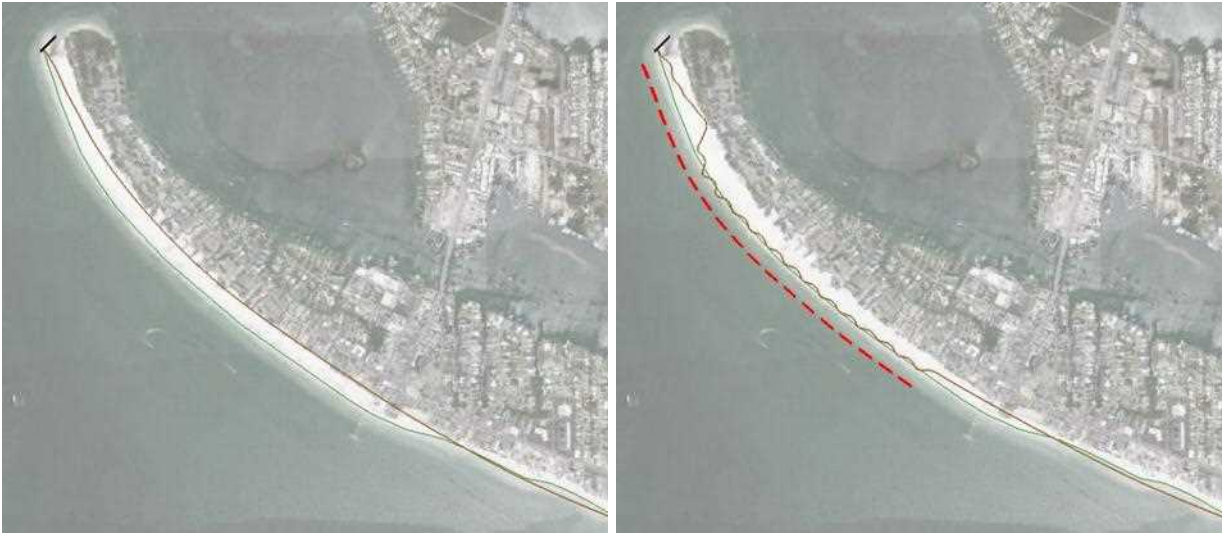
Figure 61. Beach response for Reach 1 for (left) FWOP conditions and (right) Alt 1.3 after 15 years. Green line represents the shoreline at year 0, and the brown line is the shoreline at year 15.
