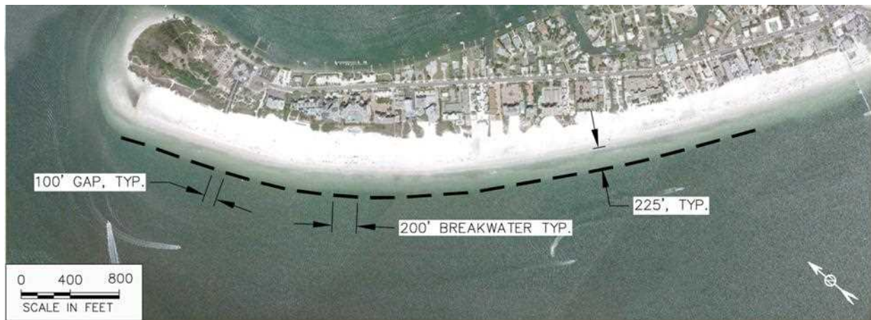
Figure 43. Planform of breakwater alternative in Reach 1 (Alternative 1.3).
