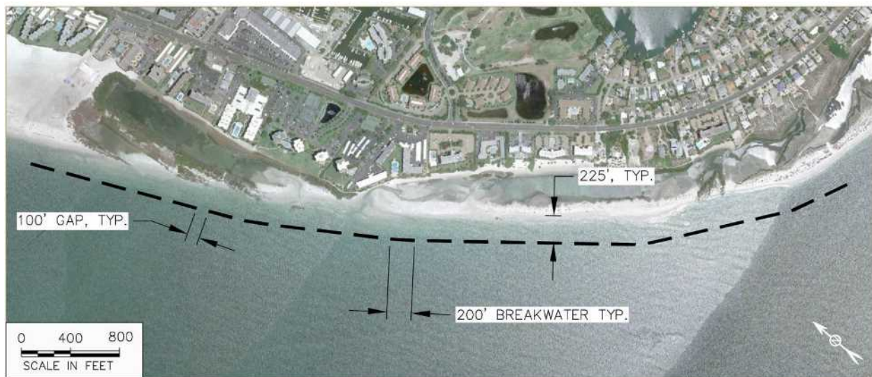
Figure 44. Planform of breakwater alternative in Reach 3 (Alternative 3.1).
