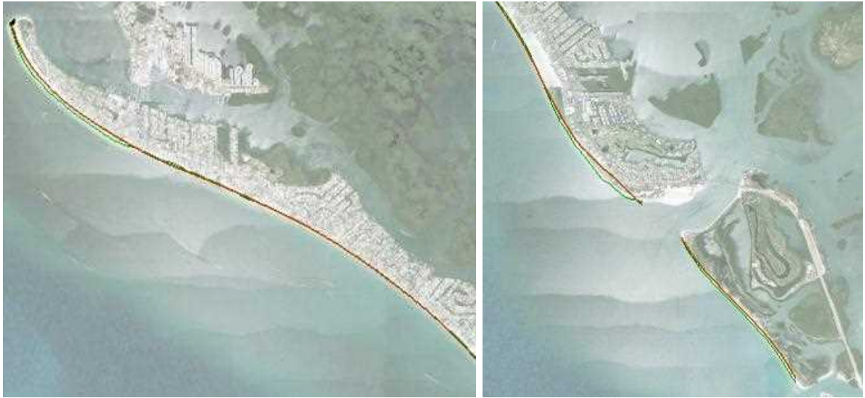
Figure 54. Beach response for FWOP conditions for the whole project shoreline after 8 years. Green line represents the shoreline at year 0, and the brown line is the shoreline at year 8.
