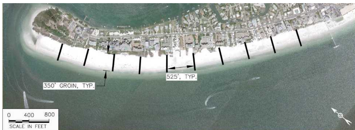
Figure 47. Planform of short groin alternative in Reach 1 (Alternative 1.2a).
