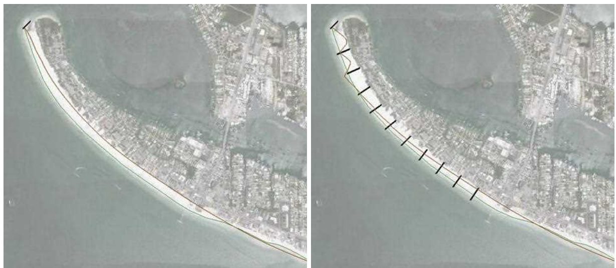
Figure 57. Beach response for Reach 1 for (left) FWOP conditions and (right) Alt 1.2 after 14 years. Green line represents the shoreline at year 0, and the brown line is the shoreline at year 14.
