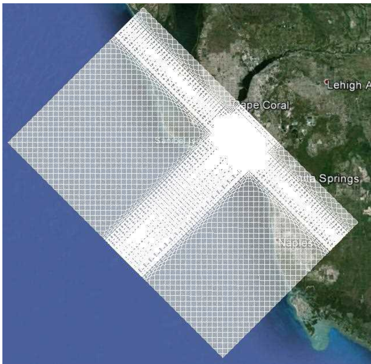
Figure 17. EI wave model domain and variable resolution grid.
