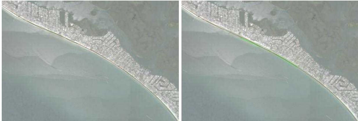
Figure 64. Beach response for Reach 2 for (left) FWOP conditions and (right) Alt 2.1 after 8 years. Green line represents the shoreline at year 0, and the brown line is the shoreline at year 8.
