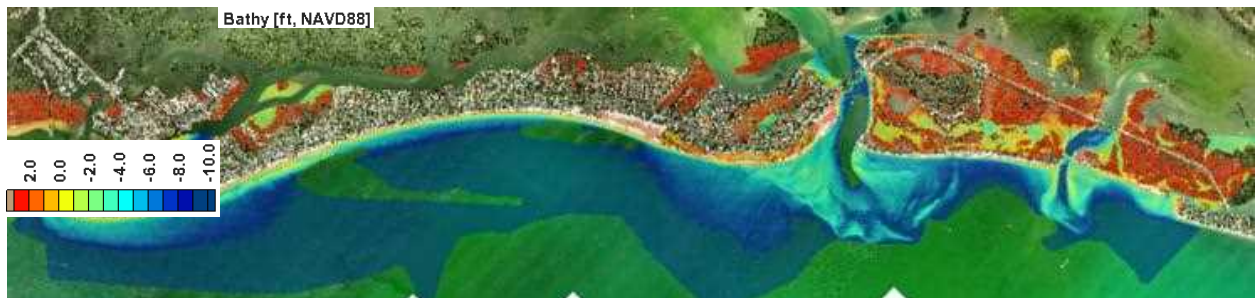
Figure 4. Bathymetric and topographic surface of project vicinity from 2010 LIDAR data set.
