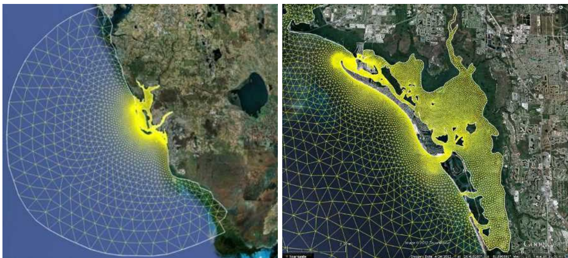
Figure 20. El circulation model domain – entire grid (left) and El project area (right).
