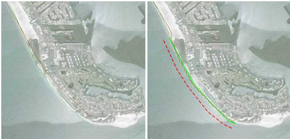
Figure 72. Beach response for Reach 3 for (left) FWOP conditions and (right) Alt 3.3 after 15 years. Green line represents the shoreline at year 0, and the brown line is the shoreline at year 15.
