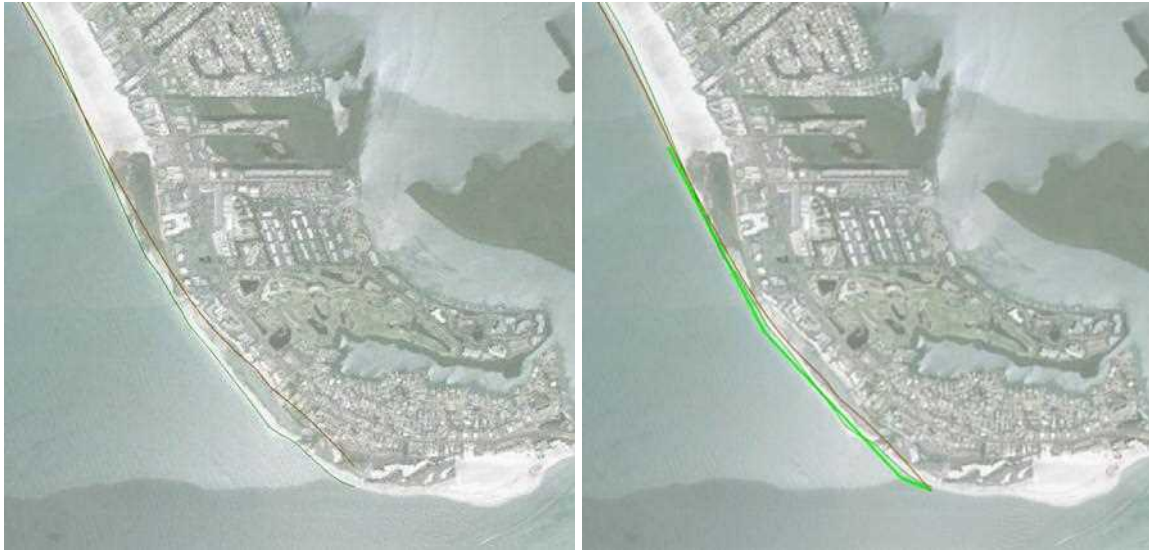
Figure 69. Beach response for Reach 3 for (left) FWOP conditions and (right) Alt 3-2 after 12 years. Green line represents the shoreline at year 0, and the brown line is the shoreline at year 12.
