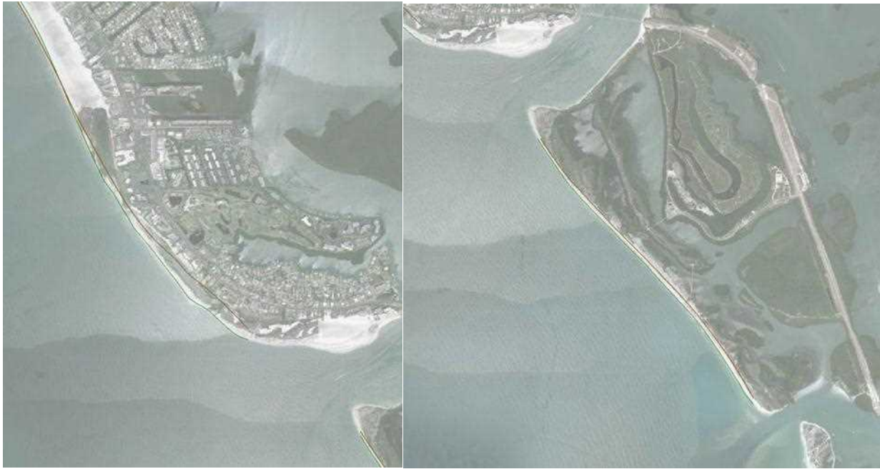
Figure 35. Beach response for FWOP conditions for (a) Reach 3 and (b) Lover's Key shoreline after 8 years
