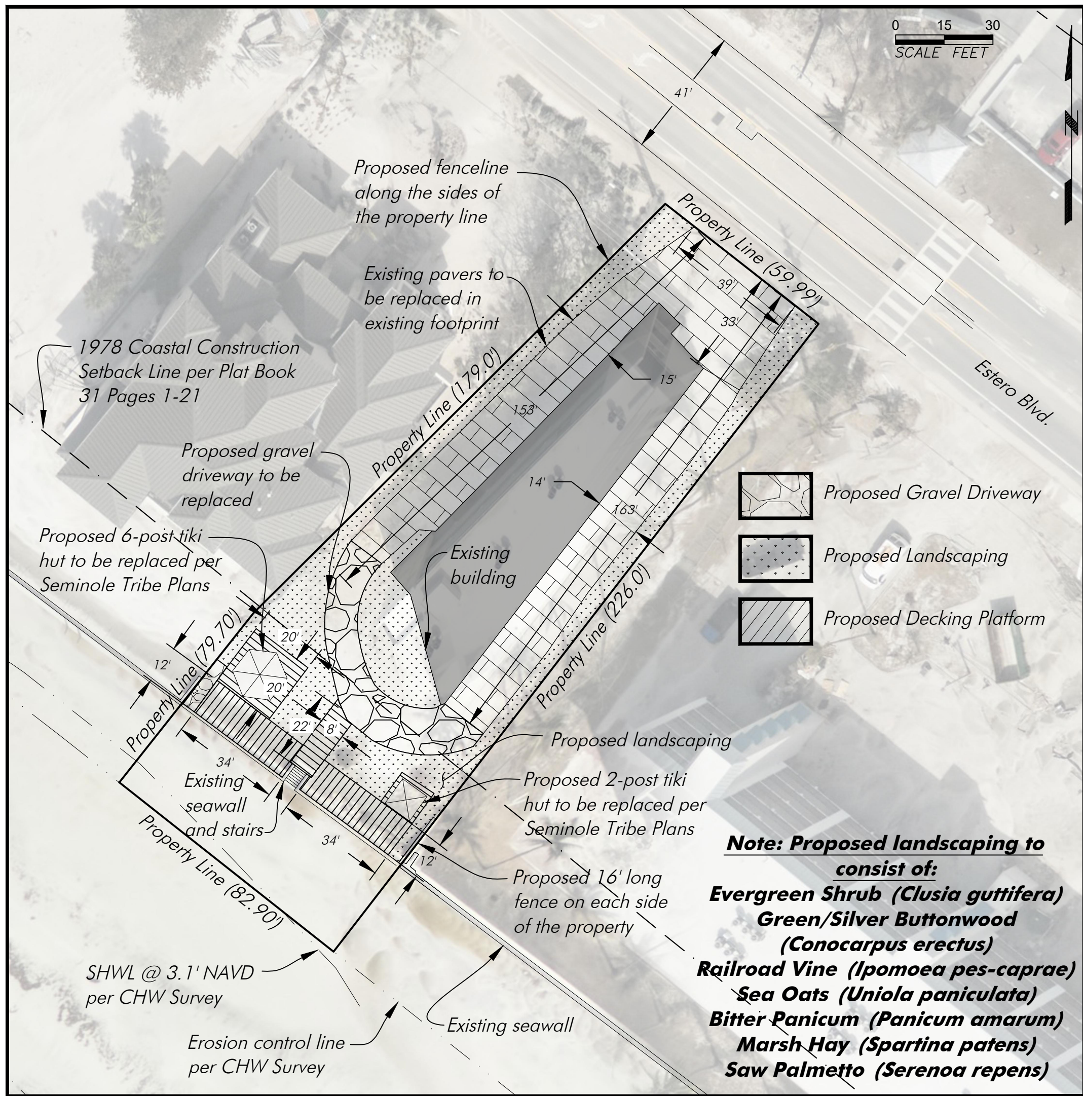
Detail A - Proposed Structures Dimension Plan Scale 1" = 30'
