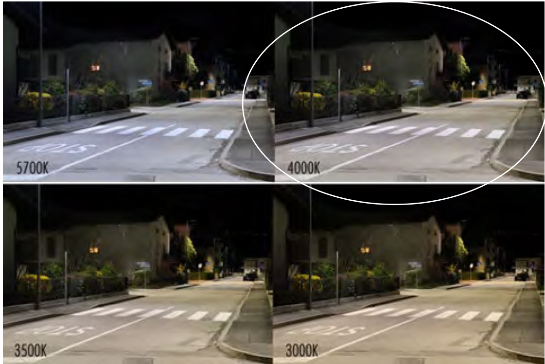
Figure 1 - 4000K is the default FDOT requirement.
