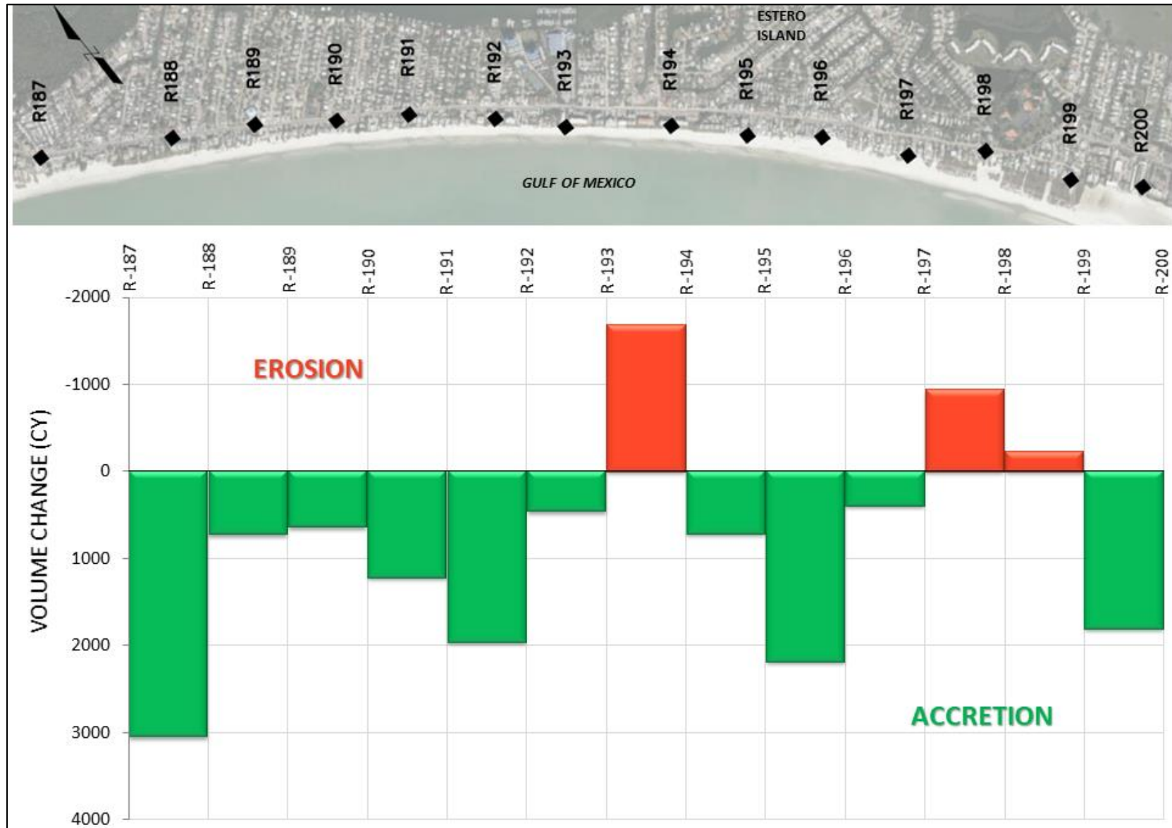
Figure 6: 2020-2021 Central Estero Island Volumetric Changes Above MHW.
